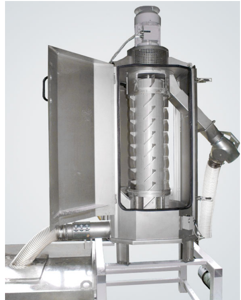
Easy access to the rotor for cleaning and servicing
