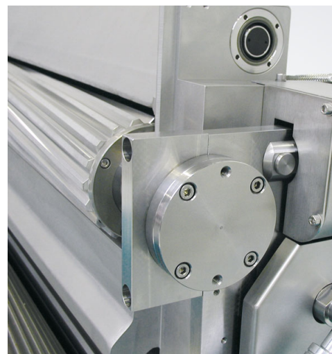
Roller bearing support outside of cutting chamber
